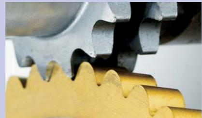
Rolling of a chain sprocket gear
