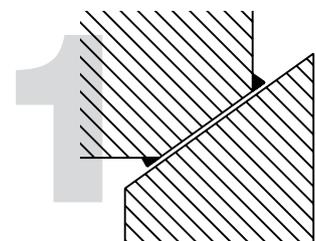
Secondary burr during chamfering
