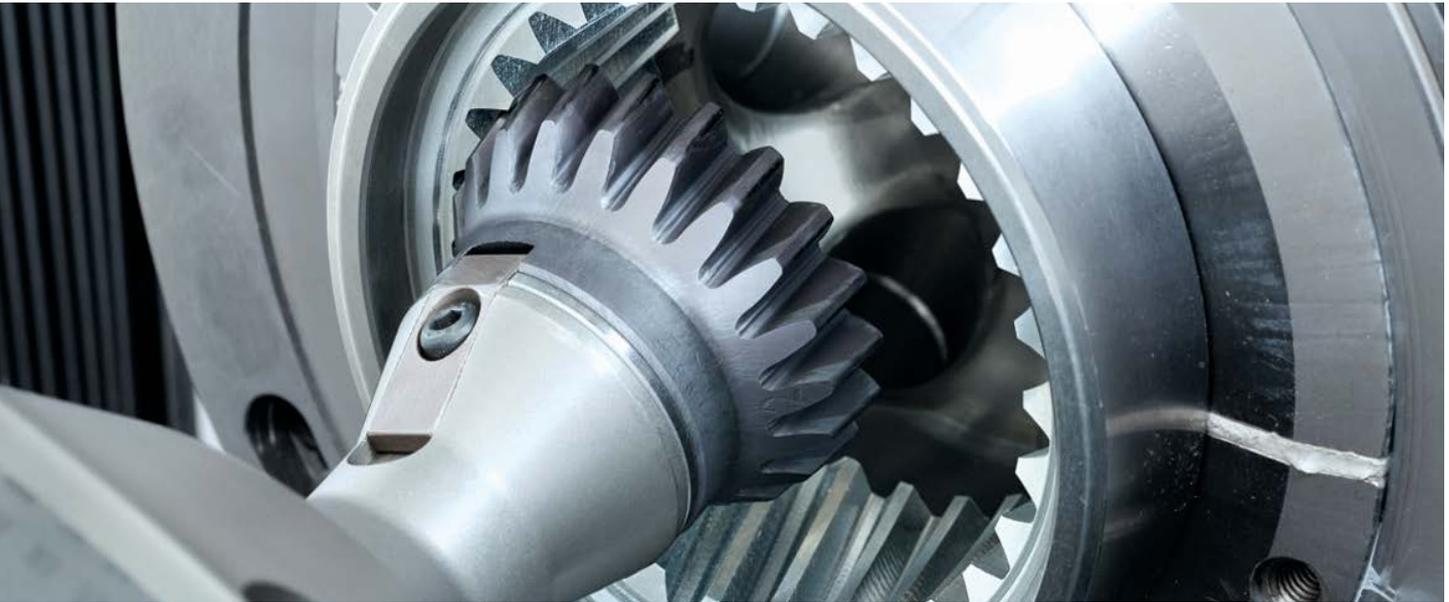
Star SU and Profilator have formed an alliance to manufacture Scudding® tools for the global market. Scudding® is a continual gear cutting process which makes both the production of external and internal gears, as well as spur and helical gearing possible.
