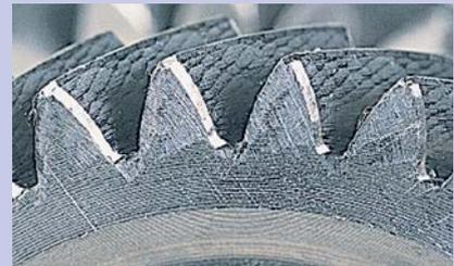
Workpiece after chamfering and deburring
