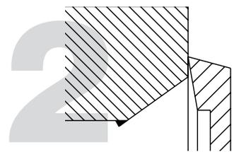
Deburring the secondary burr on gear lateral surfaces
