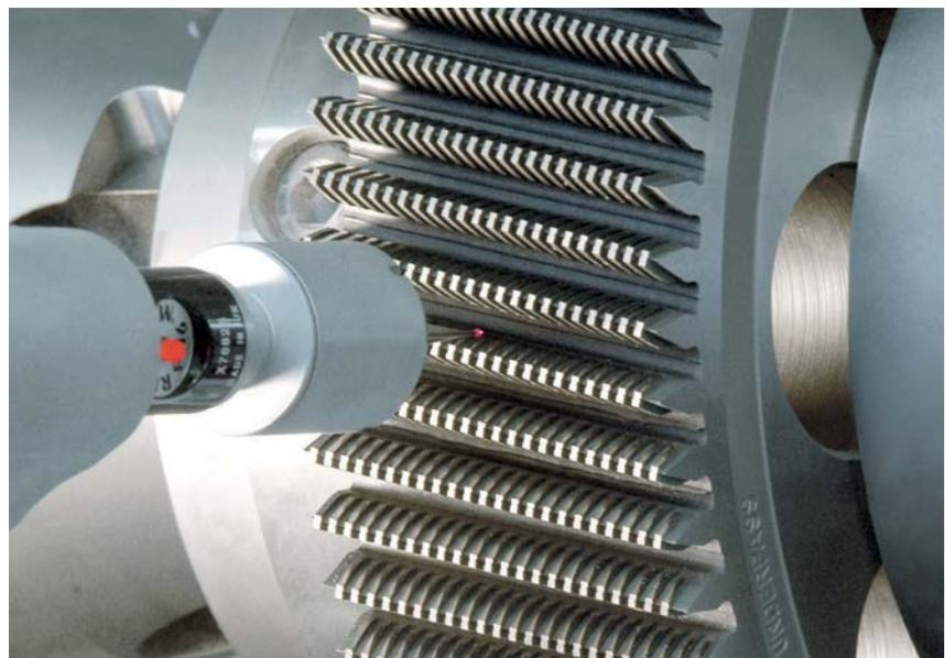
Sharpening and in-machine measurement of shaving cutters
