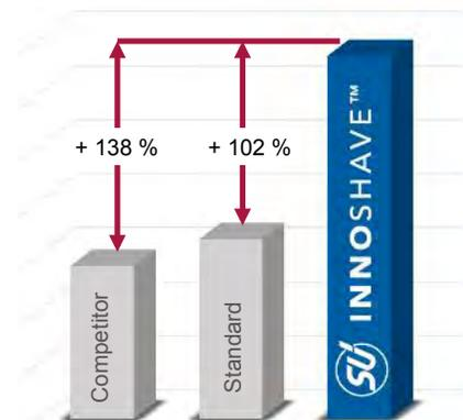
The recent improvements were shown in the reported test results. The graphic shows the result of a shaving application on a module  $m_n = 2$  mm automotive gear.
